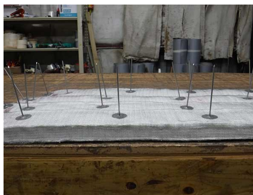
Custom door gasket for the heat treat industry
